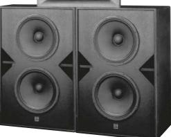
The Screen 6 full-range system has been developed for use in large to very large-scale cinema environments. The system consists of a 4 x 15" (380mm) low frequency section plus a unique mid-range unit and high frequency horn which exhibits ideal pattern control across its operating range from 300Hz-20kHz. The Screen 6 is approved by Lucasfilm for use in category 3 (over 80ft in length or over 180000ft<sup>3</sup> in volume) THX
